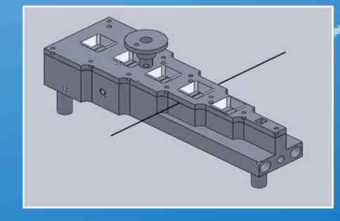
FAS17 coated (CVD) capillary flow through system:
